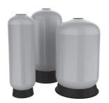
Low Profile Composite Pressure Tanks are the smart choice when space is a challenge and performance is a priority. These tanks feature a lower profile tank design with a 2 inch reduction to the top and bottom flanges, allowing the tanks to fit in tighter spaces without compromising media capacity. Their lightweight, fiberglass construction provides durability in harsh chemical environments.
